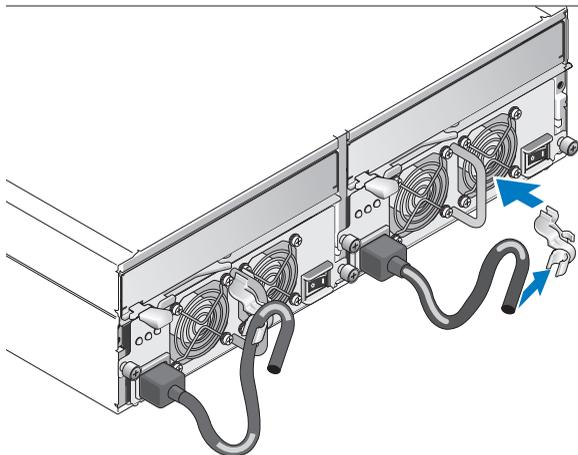
Plug the other end of the power cables into a grounded electrical outlet or a separate power source such as an uninterruptible power supply (UPS) or a power distribution unit (PDU).
